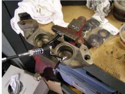
Use a lubricant (brake fluid is ok) and do not hone any more than you need. Keep the hone moving to keep things even. After honing is complete, clean the bores one more time and blow out with compressed air.
