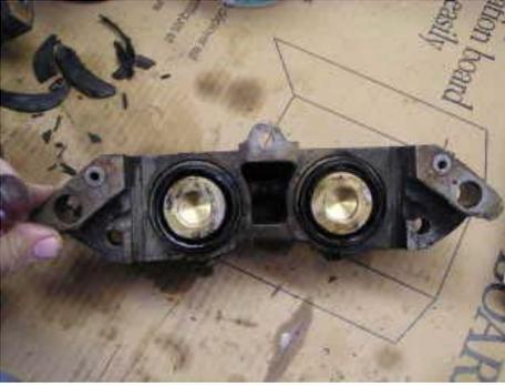
When you split the calipers the only thing to watch for is an O-ring that seals the fluid passage between the halves. The O-ring may be discarded as it will be replaced with a new one. Just note its location and fit. You may now continue with disassembly or clean the split caliper.
