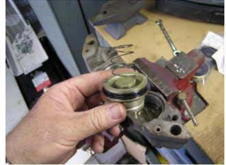
Lube the O-ring with brake fluid and work it back in the bore. Start by angling the piston in the bore and working it with an awl or similar tool. Be careful not to pinch the ring. Work it in. Do not force it.
