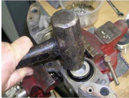
You may need to lightly tap the boot flush with the caliper housing.
