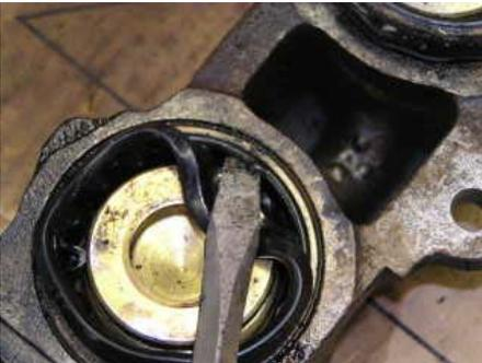
Now work the piston out of the bore. Be careful not to damage the cylinder walls.
